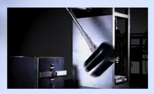
Figure 3. Example of a drop hammer for shock testing
